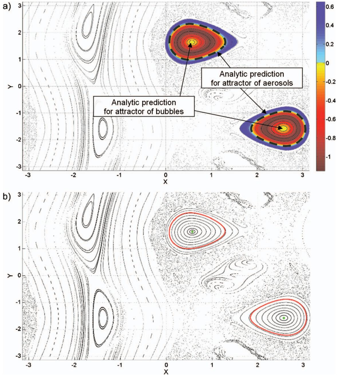
FIG. 5. (Color) (a) Poincaré map of the ABC flow. At any given point, the color refers to the computed value of  $I_T$  on the trajectory starting from that point. (b) The stream surface that attracts inertial particles obtained by the direct numerical solution of the inertial equation for  $\epsilon(3R/2-1)=-0.01$ .
