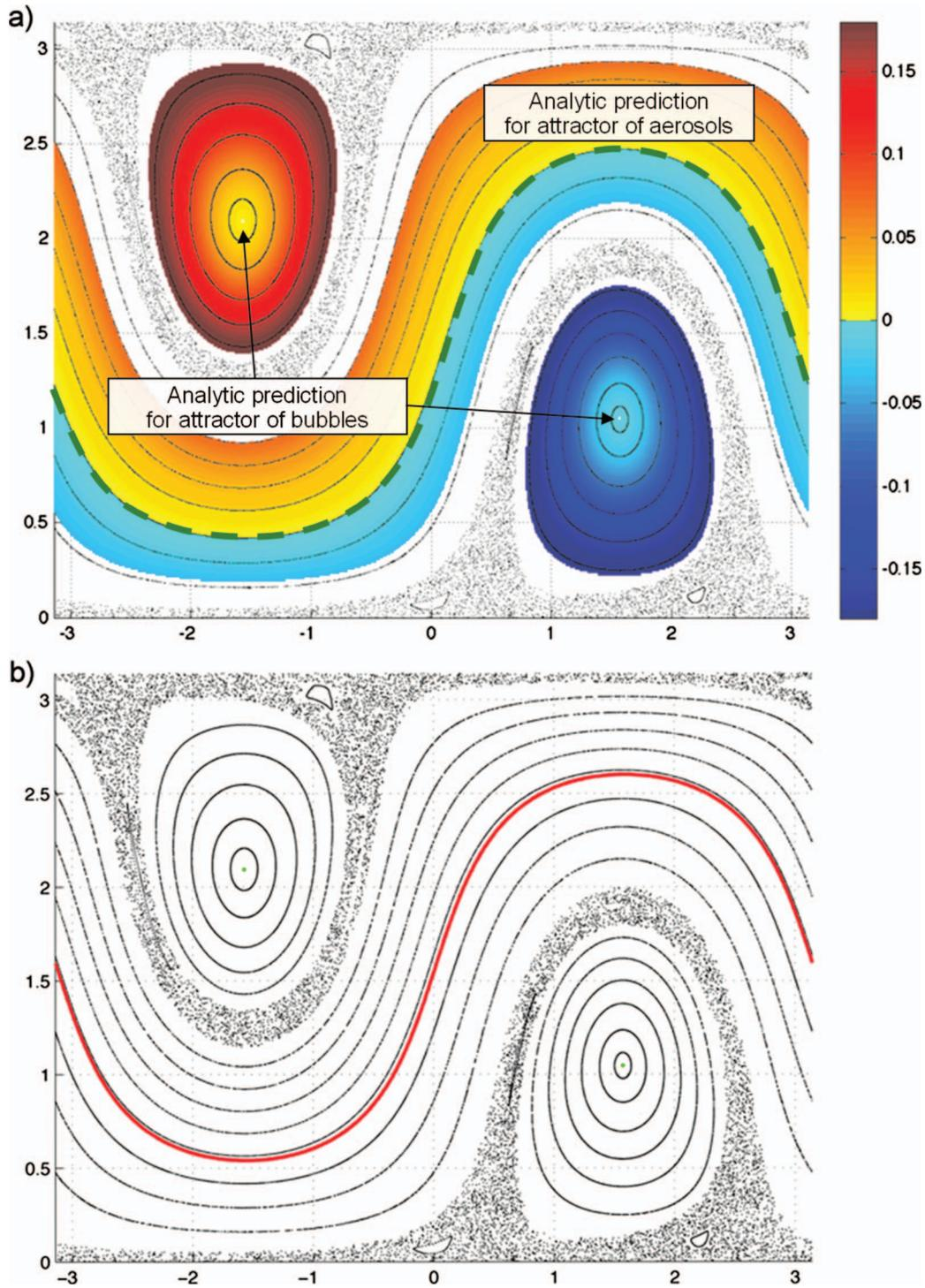
FIG. 7. (Color) (a) Poincaré map for the traveling wave in a channel with parameters  $A=1$ ,  $k=1$ ,  $c=0.5$ ,  $\sigma=0.02$ , and  $\omega=1$ ; the color refers to the value of  $I_T$  on closed stream surfaces. (b) Poincaré maps illustrating the invariant manifolds that attract inertial particles obtained from the numerical solution of the inertial equation for  $|\epsilon(3R/2-1)|=0.01$  and for both aerosols (red dots) and bubbles (green dots).
