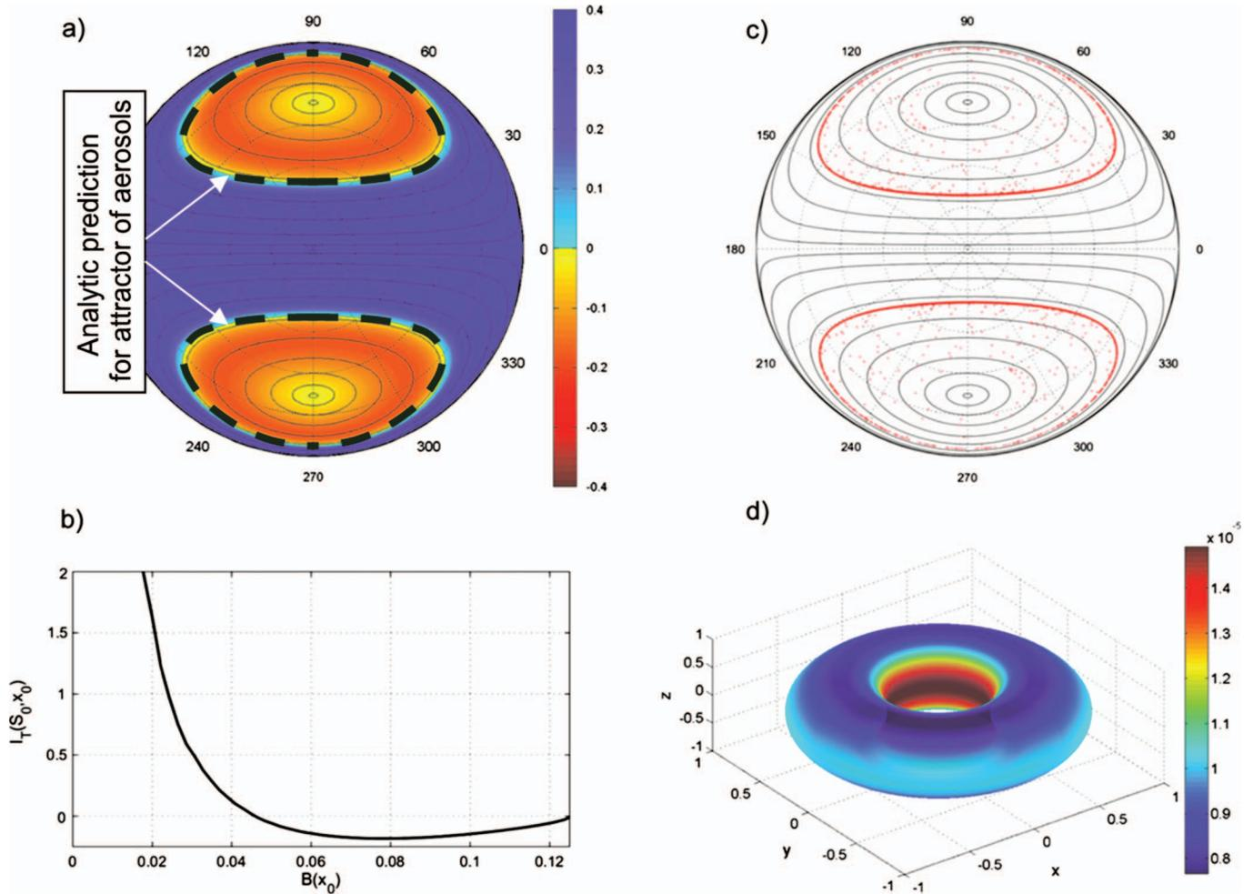
FIG. 3. (Color) (a) Poincaré section at  $x=0$  of the Hill's spherical vortex for  $c=0.15$ . The color map represents the values of the functional  $I_T(S_0, \mathbf{x}_0)$ . (b)  $I_T(S_0, \mathbf{x}_0)$  as a function of  $B(\mathbf{x}_0)$  for  $c=0.15$ . (c) Poincaré map of an inertial particle trajectory computed using the inertial equation (5). (d) Persistent stream surface for inertial particles.
