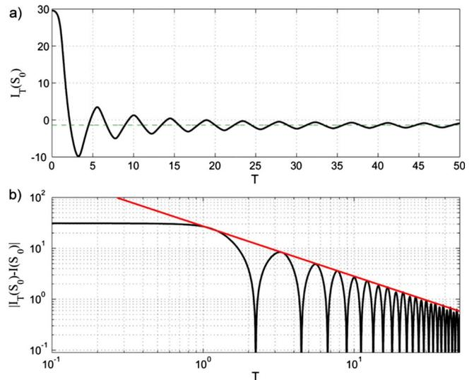
FIG. 1. (Color online) (a) Time series of the nonlinear functional  $I_T(S_0, \mathbf{x}_0)$  for  $c=0$  and initial condition  $\mathbf{x}_0=(0.7216, 0, 0)^T$ . (b) Rate of convergence of  $I_T(S_0, \mathbf{x}_0)$ .
